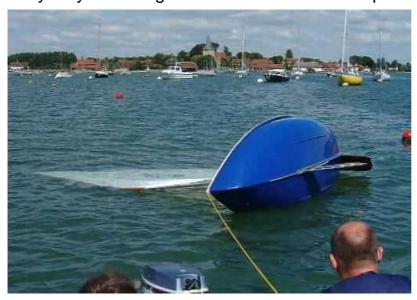
It may have been possible to simply climb down from the windward side to stand on the centreboard and right the scow very quickly.
