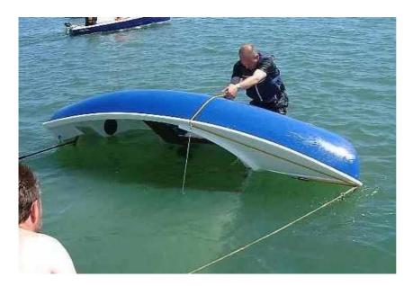
Here the painter can be seen led inside a shroud. As the rig emerges from the water the scow should right rather quickly. The crew should then climb aboard from his/her position at lowest part of the side.
